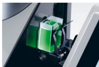
Measurement of liquids in transmission
